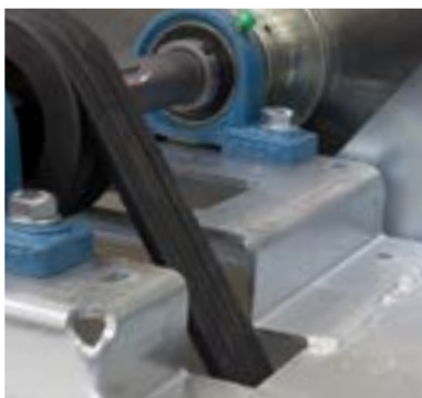
Indirect drive via triple V-belt
